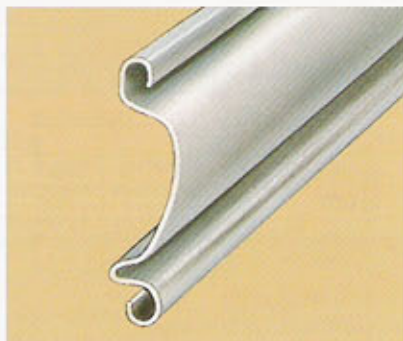
No. 2 —Curved-faced single crown slat is available in up to 20 gauge steel or to 16 B&S gauge aluminum. Depth of crown: \frac{1}{2} ", 1\frac{1}{2} " on centers.
